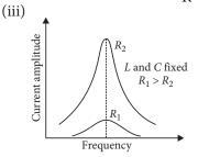
(iv) Sharpness of resonance: It is defined as the ratio of the voltage developed across the inductance (L) or capacitance (C) at resonance to the voltage developed across the resistance (R).
